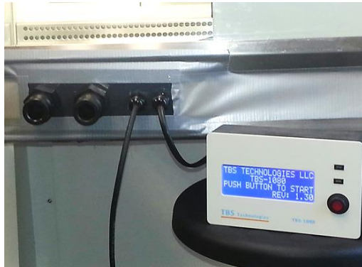
Standard Mounting Plate with Cable Glands and Banjo Fittings
